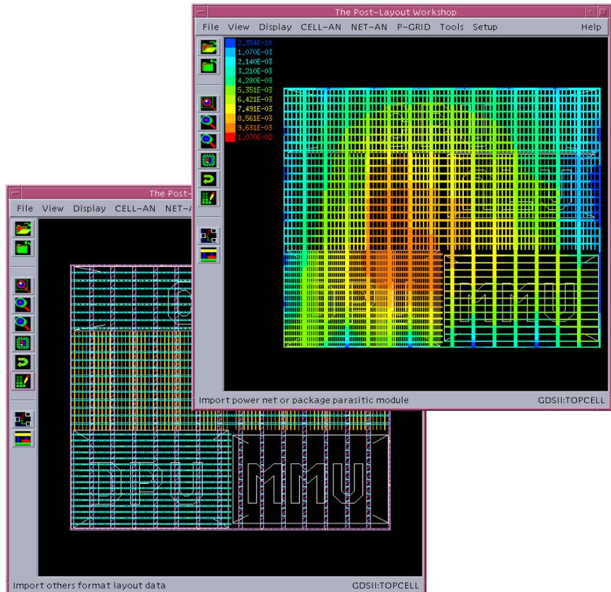
P-PLAN is a VLSI power distribution network hierarchical floorplanning tool used with P-GRID for optimizing the geometric configuration of VDD and VSS rings, internal power rails, and ring voltage source pad locations using estimated block current sources. By allowing a fast means to iterate by redefining and reanalyzing the planned power rail configuration in the floorplanning stage of the design, major electromigration and IR drop failures can be avoided.
