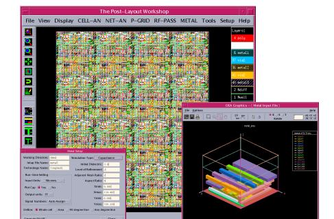
METAL is not just one program, but a collection of easy-to-use, fast, and extremely accurate programs for two and three-dimensional modeling of interconnect parasitics from integrated circuits, printed circuit boards, multi-chip modules and hybrids.
