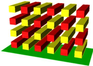
**Figure 1: A cross section of the MMCC device described in this paper. Colors represent the two different nodes of the capacitor. The bottom plane represents the substrate ground.**
