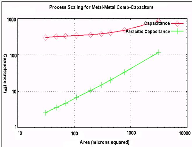
Figure 2: Effect of scaling on capacitance and parasitic capacitance.
